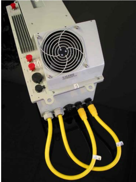
Example: 25 Watt Ku-Band Transceiver with +12V DC option installed
