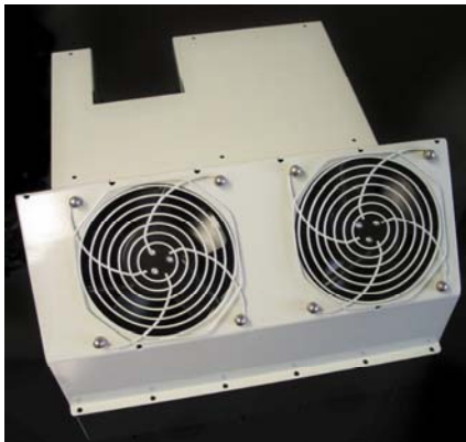
Figure 7 - Fan shroud removed from ODU
