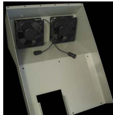
Figure 8 - Underside of fan shroud
